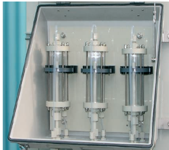
Preconditioning panel, custom built by engineers at our facility in Schiedam, The Netherlands.
