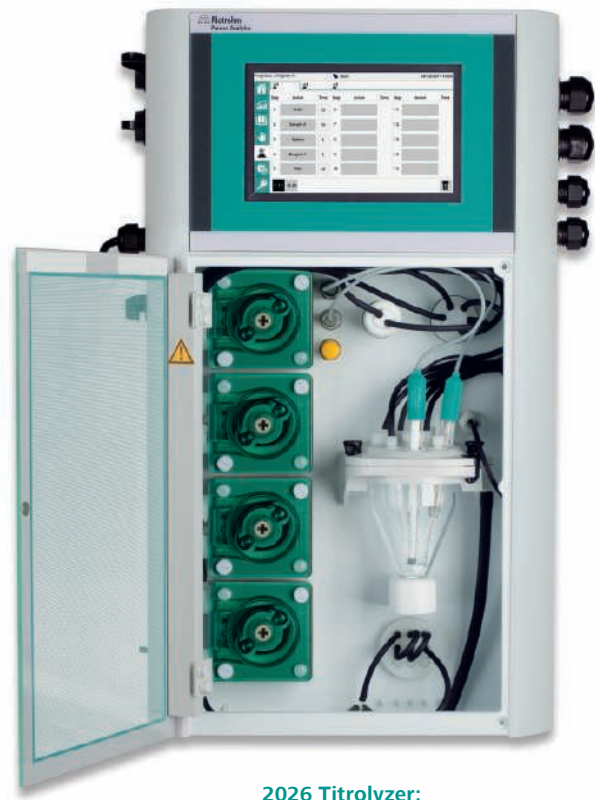
2026 Titrolyzer: configured to monitor water hardness
