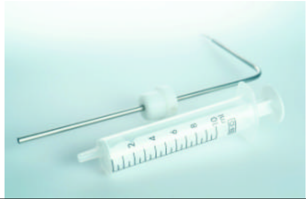
PT-MDS Manual Sampling System includes sampling tubes, disposable syringes and 10 micron filters
